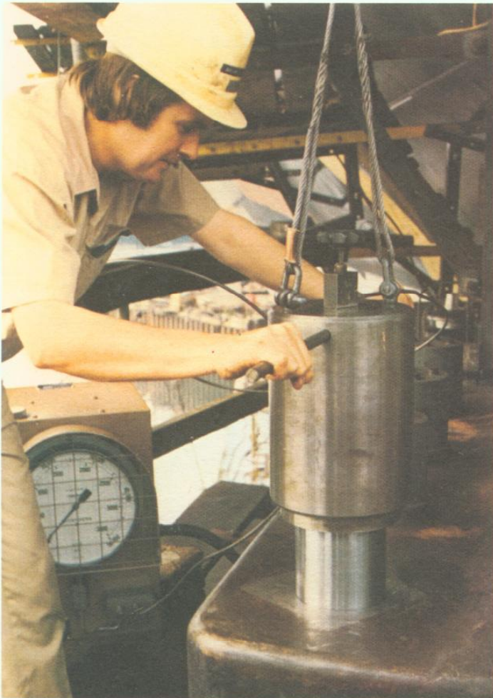
ABOVE A Moorside sales engineer positioning a Morgrip bolt to fix a ship's rudder at a shipyard on Tyneside
