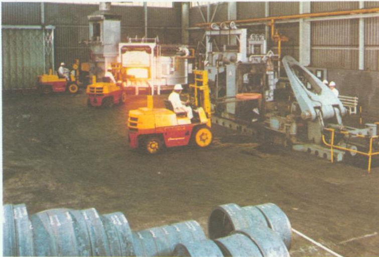
ABOVE The 1500 ton hydraulic press at Sheffield has a high output due to the forging manipulators and furnaces in the shop
