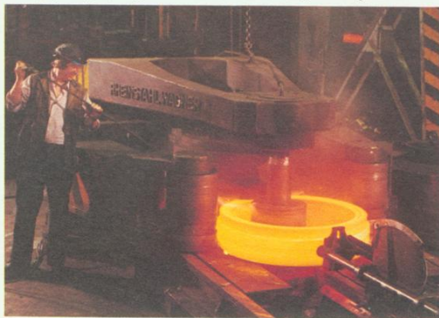
BELOW Blaenavon's speciality since 1967 has been the profile rolling of rings up to 3 metres diameter in aerospace alloys
