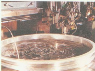
A titanium alloy ring, destined for a jet engine is machined at Blaenavon before final testing
