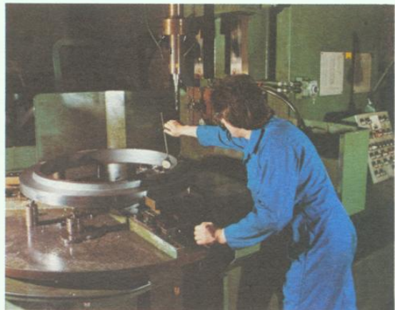
ABOVE Automatic and precisely spaced drilling of flange bolt holes is done on this specialised machine by John Brereton & Co. Ltd at Oldham
