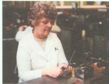
ABOVE Hollow turbine blades are checked dimensionally at every step in manufacture at Moorside
