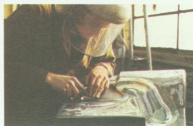
ABOVE The die for a tractor steering arm nears completion in Whittingham & Porter's die shop
