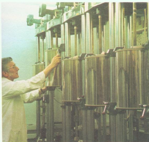
Approval of forgings in high nickel-base alloys involves stress rupture testing at elevated temperatures in Birley House laboratories
