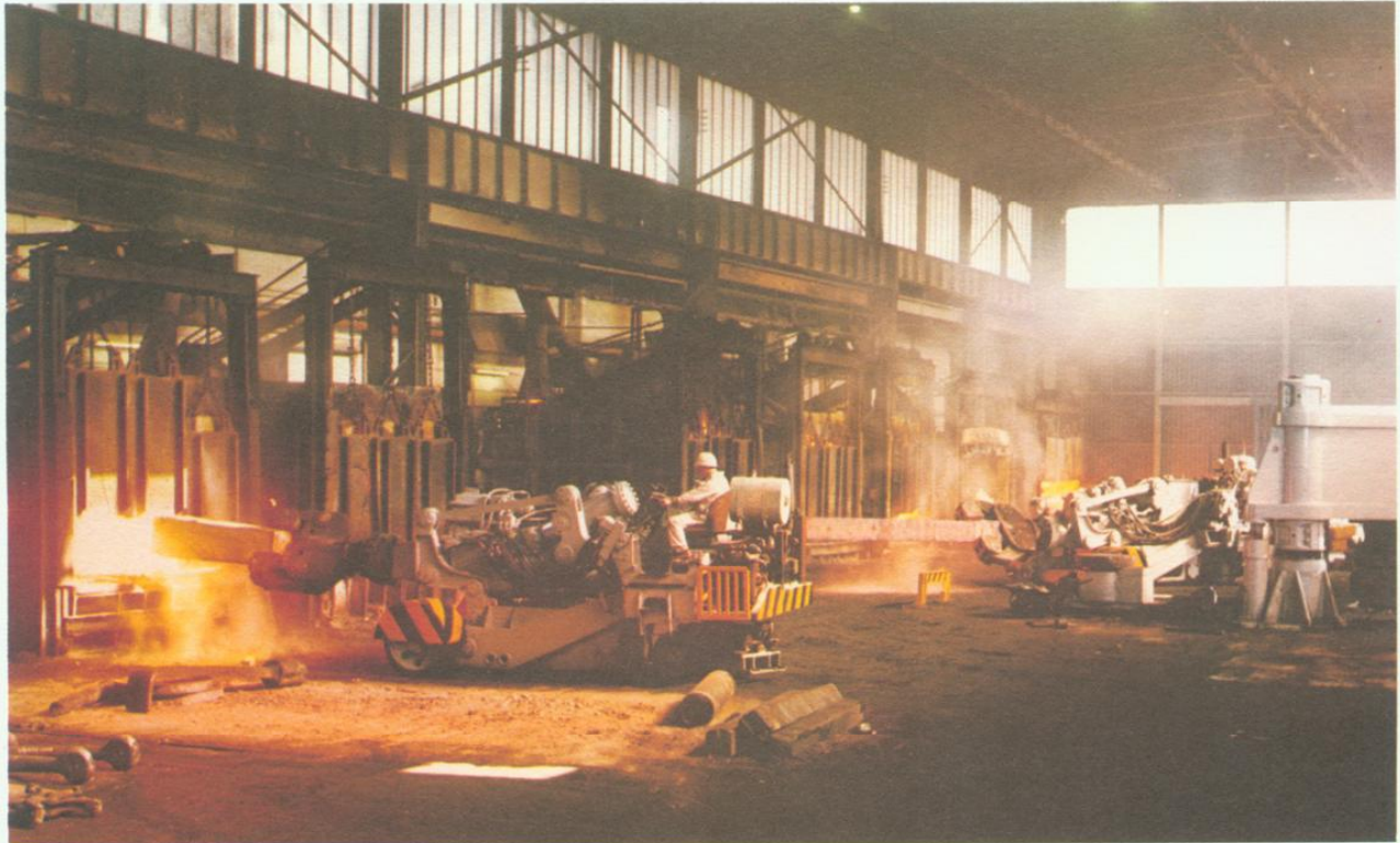
ABOVE The 1500 ton hydraulic press at Sheffield has a high output due to the forging manipulators and furnaces in the shop
