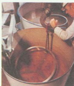
Aerospace components require a series of non-destructive tests after forging, including ultra-sonic immersion crack detection
