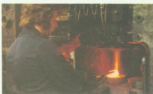
ABOVE A diesel rocker arm starts its forging process on a Whittingham & Porter Press
